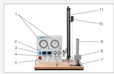
1 precision manometer, 2 controller, 3 230VAC connection, 4 connections for current signals, 5 DC voltage source, 6 pressure regulator, 7 fixture for control loop components, 8 connection for low pressures, 9 assembly tube for control loop components, 10 heightadjustable tank, 11 level tube with scale for low pressures
