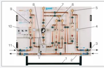
1 frame, 2 panel, 3 water connections for heating system, 4 bimetallic thermometer, 5 bleed valve, 6 differential pressure overflow valve, 7 pump, 8 three-way mixing valve with actuator motor, 9 rotameter, 10 mixing valve controller switch cabinet, 11 water connections for boiler
