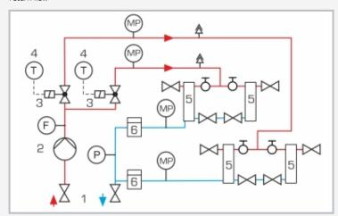
Heating circuit with two subcircuits
