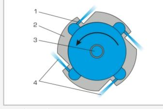
Principle of operation of the reaction turbine rotor 1 outlet nozzle, 2 turbine rotor, 3 compressed air inlet, 4 exiting air flow
