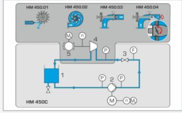
1 tank, 2 pump, 3 flow control valve, 4 turbine, 5 brake, M motor; F flow rate, P pressure, n speed,  $M_{\rm d}$  torque
