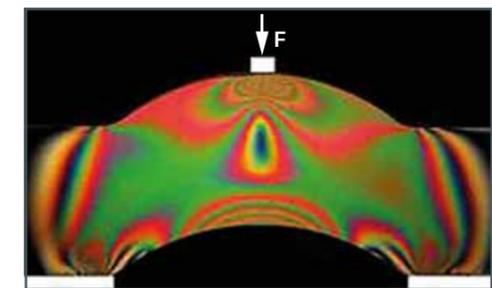
A polariscope can be used to study transparent models of components, whose optical properties change under the influence of internal stresses. If the model is stress-free, there is no birefringence and the model appears black. If a load is applied and increased, this creates a path difference that increases in proportion to the magnitude of the difference in the principal stresses.
