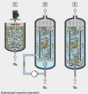
${\bf C}$  stirred tank reactor,  ${\bf D}$  jet reactor,  ${\bf E}$  airlift reactor
