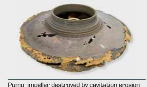
Pump impeller destroyed by cavitation erosion
