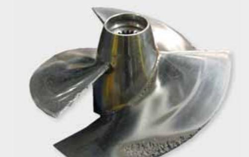
Ship's propeller destroyed by cavitation erosion
