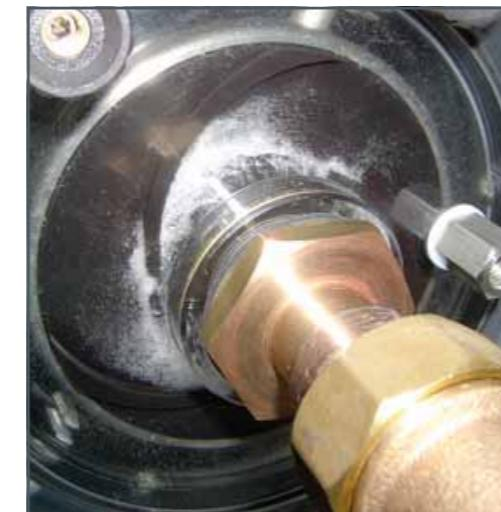
Formation of vapour bubbles due to cavitation at a pump impeller (HM 380)
