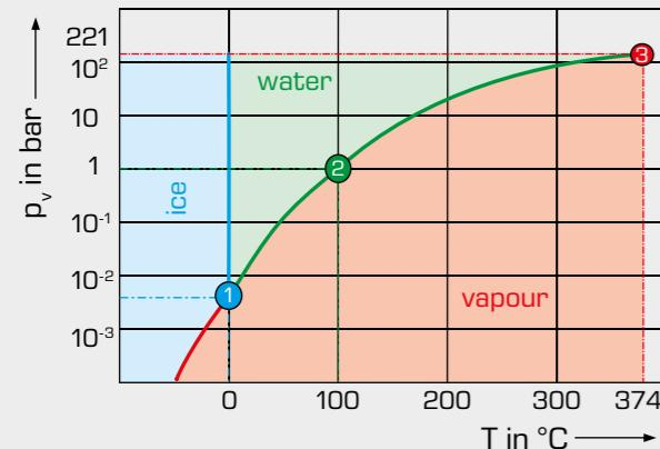
Temperature-pressure diagram of water
