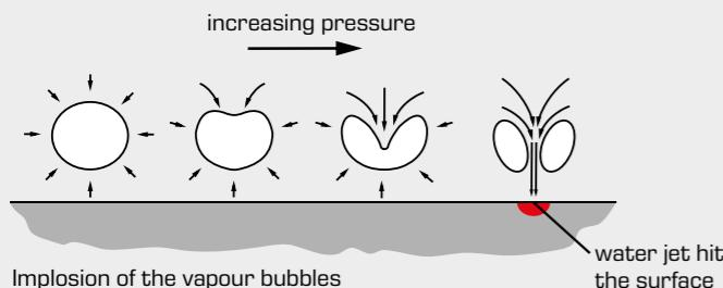
Implosion of the vapour bubbles
