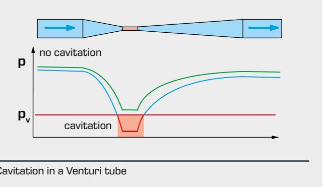
Cavitation in a Venturi tube
