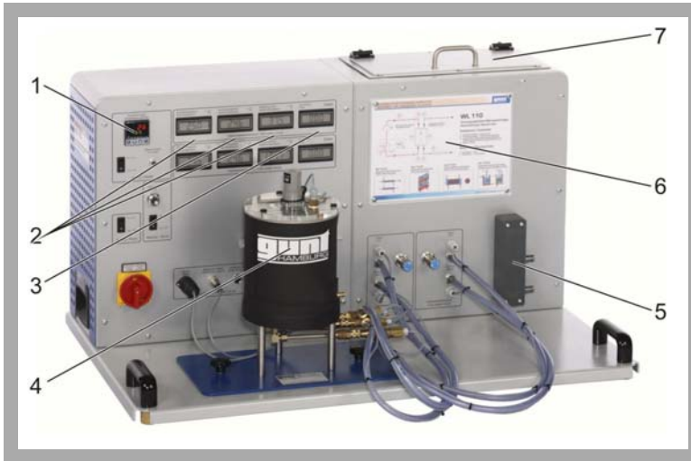
1 temperature controller, 2 temperature displays, 3 flow rate displays, 4 jacketed vessel with stirrer and coil WL 110.04, 5 cold water circuit connections, 6 process schematic, 7 hot water tank
