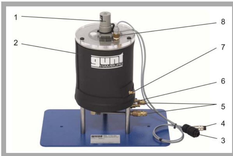
1 stirring machine, 2 tank, 3 stirring machine connection, 4 temperature sensor connection, 5 water outlet and inlet in tank, 6 coiled tube water connection, 7 jacket water connection, 8 temperature sensor
