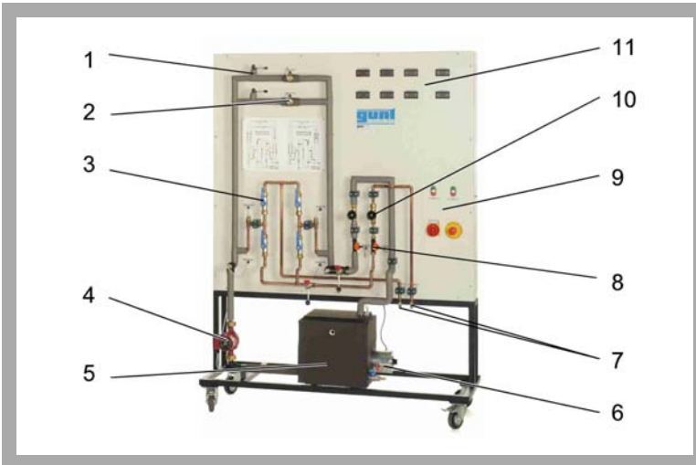
1 vent valve, 2 temperature sensor, 3 ball valve, 4 pump, 5 tank, 6 heater with thermostat, 7 water connections, 8 flow rate sensor, 9 main switch and emergency, pump and heater switches, 10 valve to adjust flow rate, 11 displays
