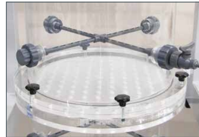
Sampling point within the trickling filter
