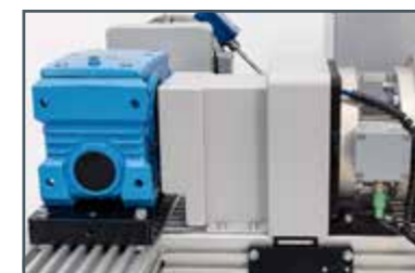
mechanical protection, output shaft/clutch, load side
