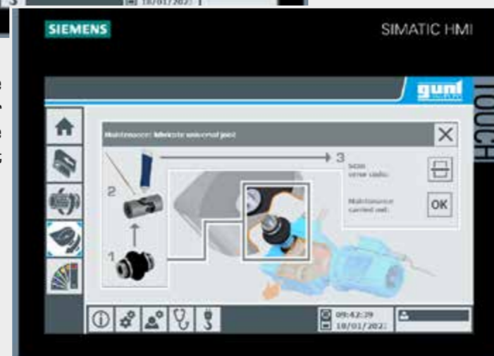
maintenance steps for lubricating the shaft joint
