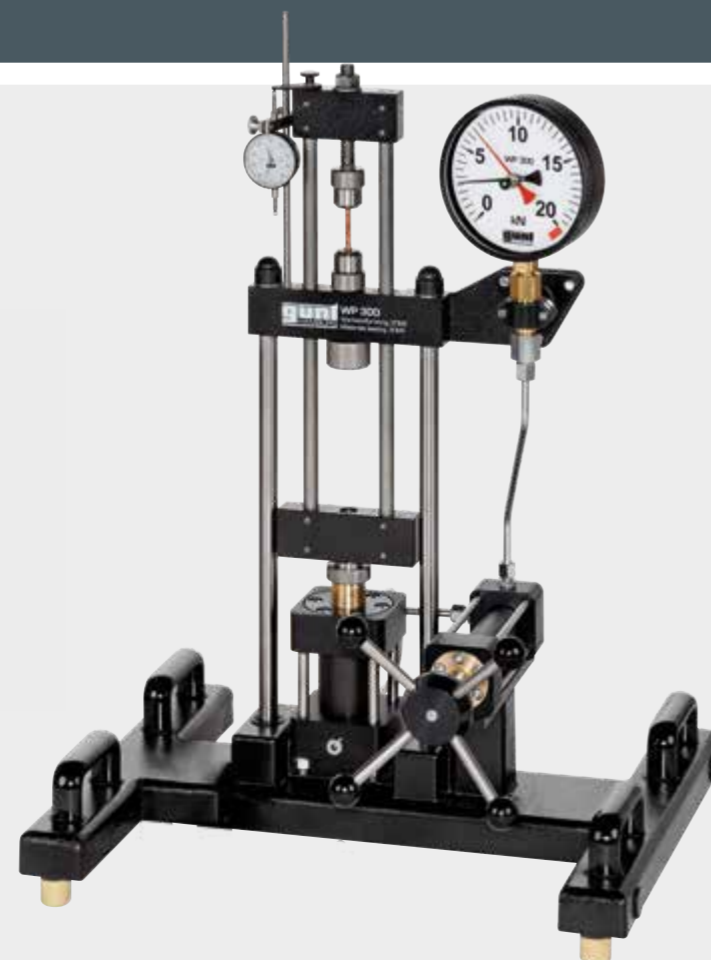
Tensile specimens with circular cross-section according to DIN 50125, material: Al, Cu, St, CuZn
