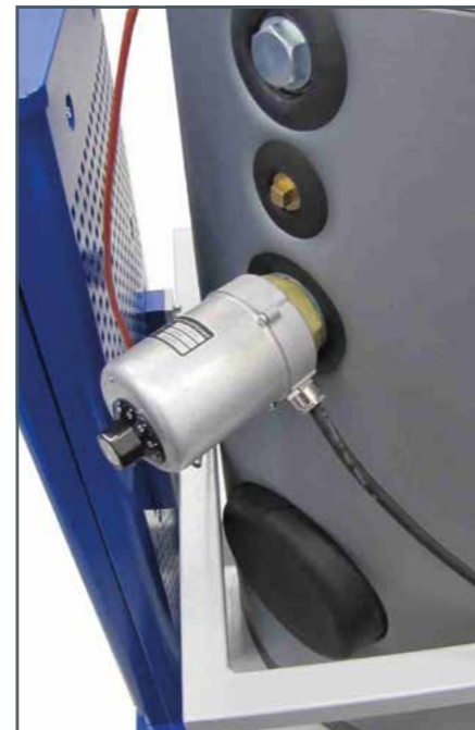
The storage tank is emptied in preparation for the experiment. The auxiliary heater can easily be inserted subsequently in just a few steps.
