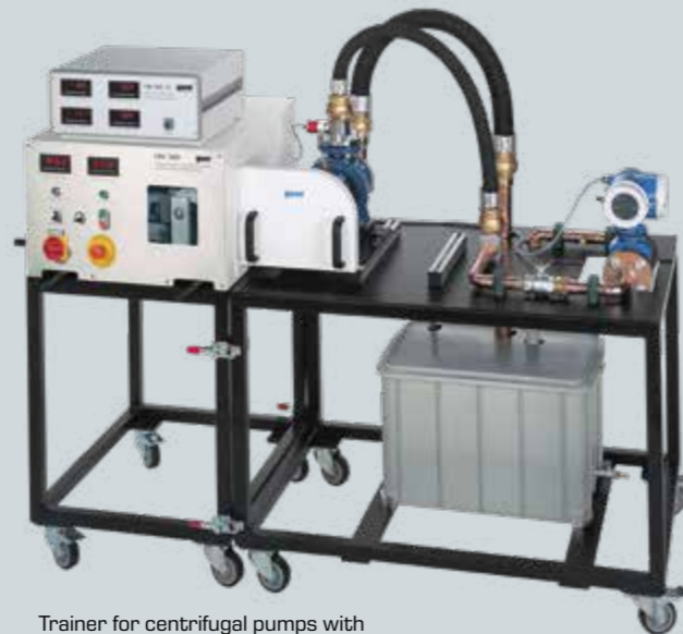
Trainer for centrifugal pumps with supply unit HM 365.10, centrifugal pump HM 365.11 and drive unit HM 365
