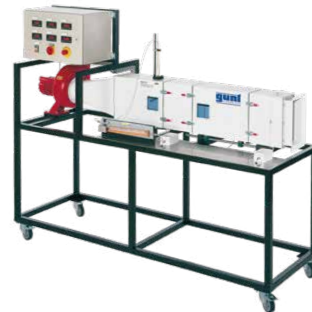
WL 312 Heat transfer in air flow Convective heat transfer using shell & tube and finned tube heat exchangers
