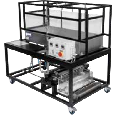
HM 141 Hydrographs after precipitation Correlations between precipitation and seepage; various drainage methods
