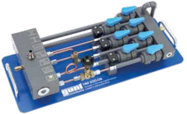
HM 250.09 Fundamentals of pipe friction Pipe friction for laminar/turbulent flow, Reynolds number and pipe friction factor
