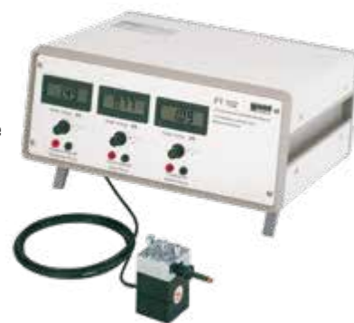
FT 102 Cutting forces during turning Measuring the forces acting on a lathe tool; three-component force measuring device
