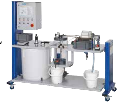
CE 286 Nutsche pressure filter Discontinuous cake filtration by positive pressure
