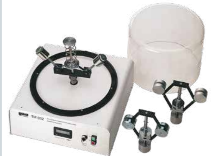
TM 632 Centrifugal governor Characteristic curves of different centrifugal force governors
