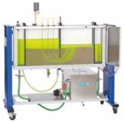
HM 169 Visualisation of seepage flows Graphical determination of flow nets; investigation of water pressure on structures
