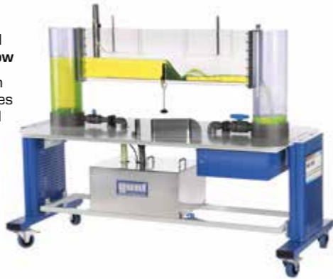
HM 111 Pipe networks Pressure losses at various piping elements and pipe networks; parallel and series connection of pipe sections
