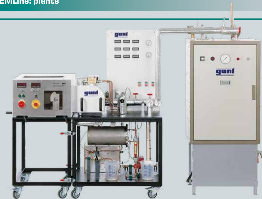
Experimental plant with two-cylinder steam engine ET 813, steam generator ET 813.01 and brake unit HM 365
