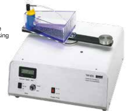
TM 632 Centrifugal governor Characteristic curves of different centrifugal force governors
