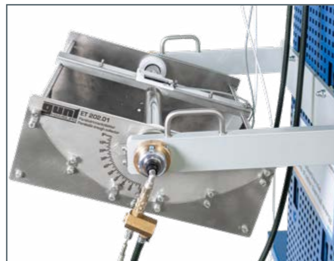
pivoting parabolic trough collector
