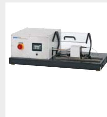
The WP 510 experimental unit generates reference moments of 200Nm
