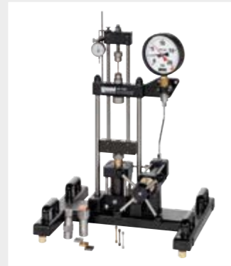
The compact WP 300 experimental unit generates a 20kN test load
