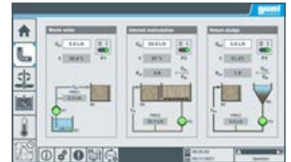
Touch screen: operation of the pumps
