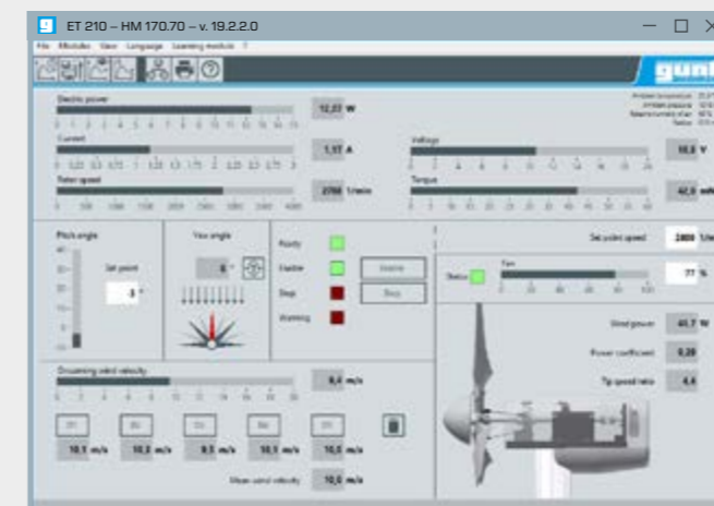
GUNT software for unit control and measurement data acquisition via PC
