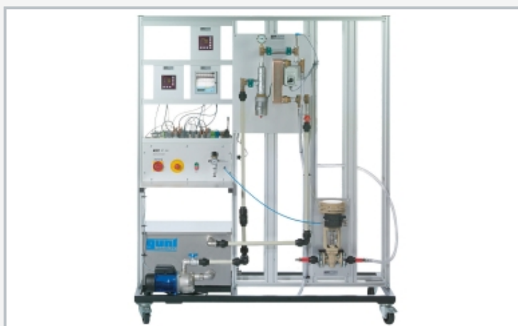
The illustration shows the layout of a temperature control system. In addition to the base module RT 450, it includes the following components: RT 450.04 (controlled system module: temperature), RT 450.11 (controller), RT 450.12 (recorder), RT 450.21 (control valve) and RT 450.36 (temperature sensor).
