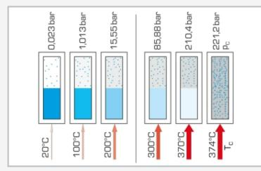
Heating up water in a closed tank: the pressure and temperature increase proportionally up to the critical point, at which fluid and vapour are no longer distinguishable from each other; critical point at  $T_c$ =374°C,  $p_c$ =221bar, line: temperature limit of the experimental unit
