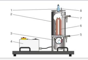
1 safety valve, 2 pressure boiler with insulating jacket, 3 Bourdon tube pressure gauge, 4 switch cabinet with temperature display, 5 drain valve, 6 heater, 7 overflow, 8 temperature sensor
