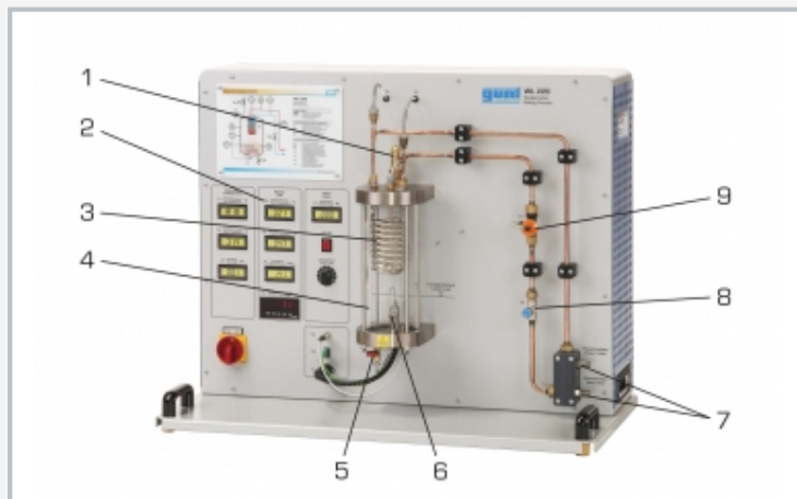
1 safety valve, 2 displays for temperature, flow rate and pressure, 3 condenser, 4 pressure vessel, 5 drain valve for the evaporating liquid, 6 heater, 7 cooling water connection, 8 valve for adjusting the cooling water, 9 cooling water flow rate sensor
