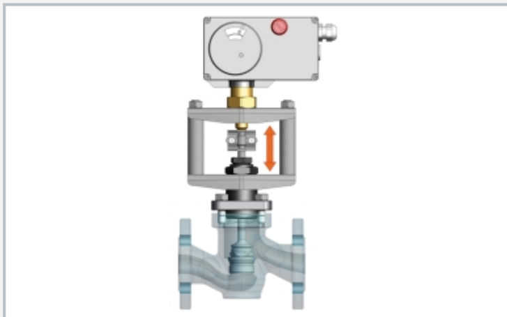
Transparent sectional view of the assembled control valve (screenshot from assembly video)
