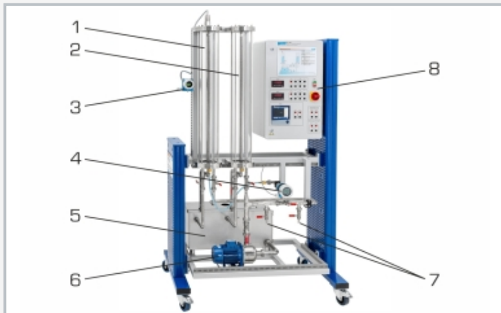
1 tank with two different sensors for level measurement, 2 tank with two free connections for own measuring instruments, 3 capacitive level sensor, 4 pressure sensor for level measurement, 5 storage tank, 6 pump, 7 external water connections, 8 switch cabinet with connection options
