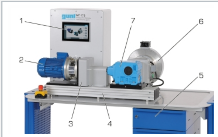
1 touch screen for operation, 2 drive motor, 3 protective cover, 4 base plate for holding motor and gear, 5 tools, 6 brake, pivoted, 7 MT 123 Spur and worm gear
