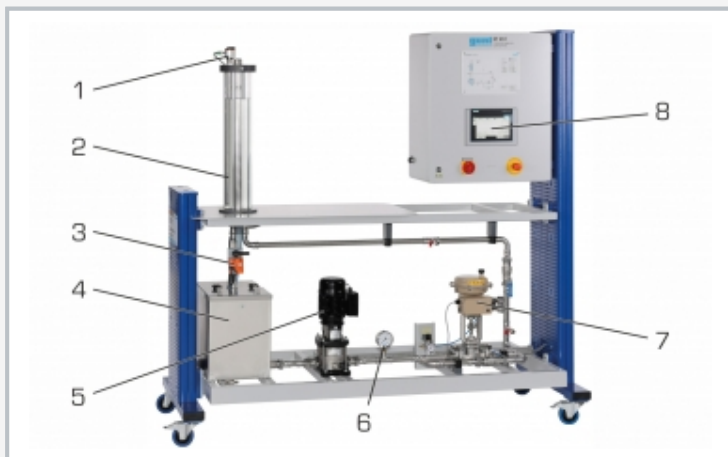
1 smart level sensor, 2 transparent tank, 3 ball valve with motor drive, 4 storage tank, 5 pump, 6 manometer, 7 control valve, 8 touch screen
