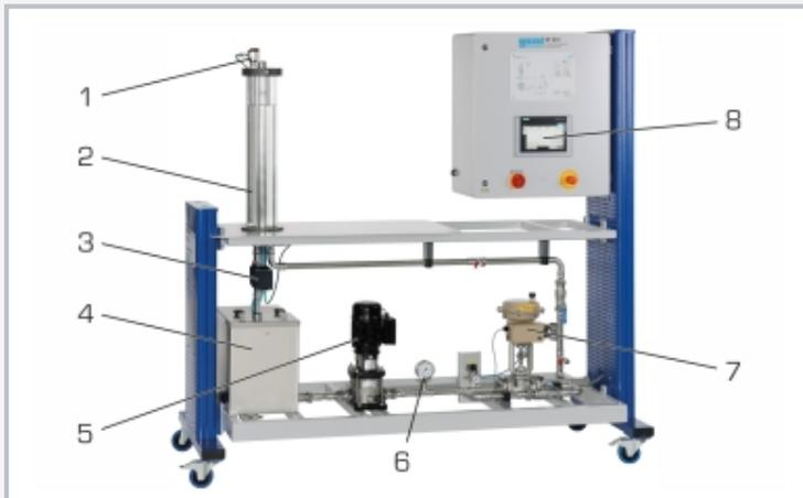
1 smart level sensor, 2 transparent tank, 3 proportional valve with motor drive, 4 storage tank, 5 pump, 6 manometer, 7 control valve, 8 touch screen
