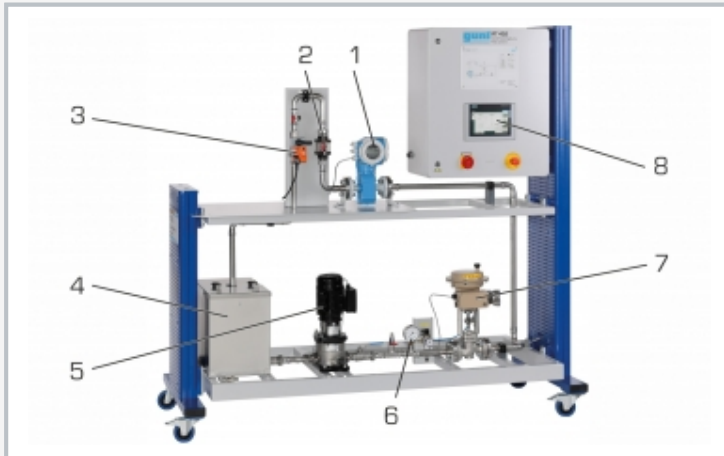
1 smart flow rate sensor, 2 flow rate indicator, 3 ball valve with motor drive, 4 storage tank, 5 pump, 6 manometer, 7 control valve, 8 touch screen
