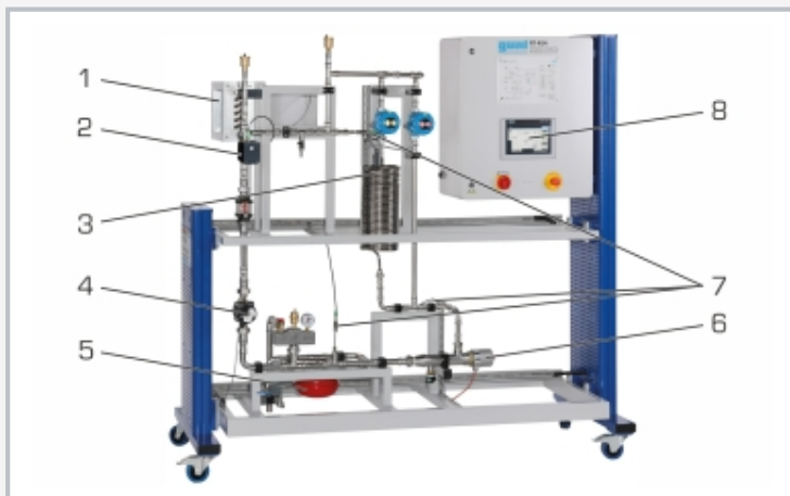
1 cooling unit (air/water heat exchanger with fan), 2 proportional valve with motor drive, 3 process delay pipe section, 4 pump, 5 expansion tank, 6 heater, 7 smart temperature sensors, 8 touch screen
