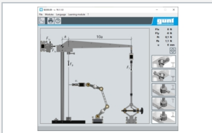
Screenshot of the GUNT software with display of measured forces and deflection
