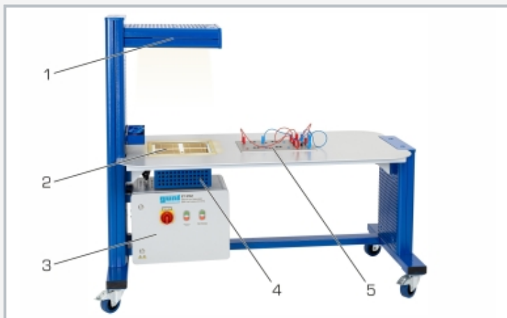
1 lighting unit, 2 four monocrystalline Si solar cells, 3 control unit, 4 Peltier module, 5 patch panel
