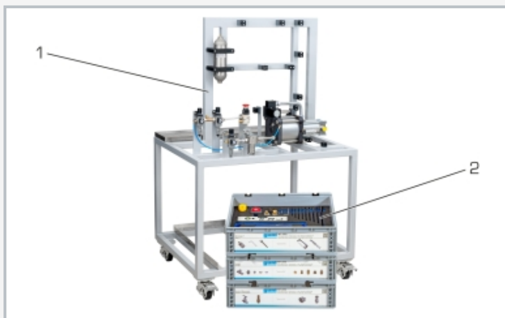
1 basic setup with pre-assembled gas booster, pressure vessel and compressed air connections on the laboratory side, 2 storage system with components, tools, spare parts
