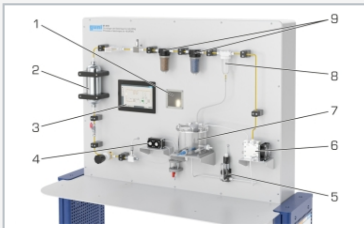
1 halogen lamp as electrical consumer, 2 buffer tank for H 2 , 3 touch screen, 4 PEM fuel cell, 5 diaphragm pump, 6 PEM electrolyser, 7 water tank, 8 water separator, 9 drying units
