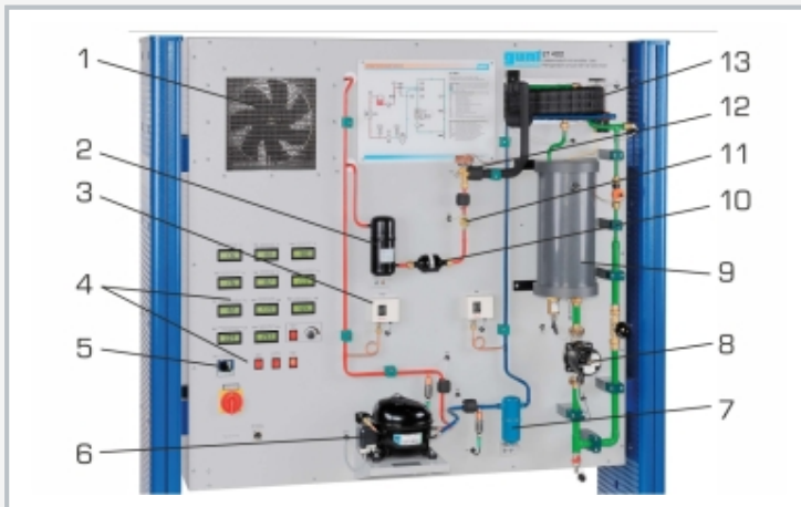
1 condenser with ventilator, 2 receiver, 3 high pressure switch, 4 displays and controls, 5 heater controller, 6 compressor, 7 liquid separator, 8 pump, 9 warm water tank with heater, 10 filter/drier, 11 sight glass, 12 expansion valve, 13 evaporator
