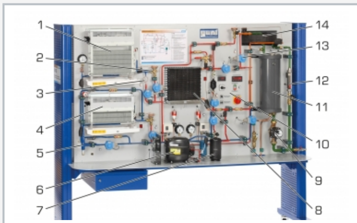
1 evaporator, 2 expansion valve, 3 capillary tube, 4 freezing stage evaporator, 5 evaporation pressure controller, 6 compressor, 7 receiver, 8 heat exchanger with fan, 9 pump, 10 display and control elements, 11 tank for glycol-water mixture, 12 flow meter (glycol-water), 13 solenoid valve, 14 coaxial coil heat exchanger
