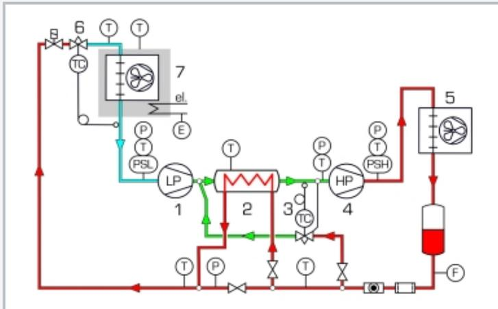
1 LP compressor, 2 intercooler, 3 reinjection valve, 4 HP compressor, 5 condenser, 6 expansion valve, 7 evaporator; T temperature, P pressure, E electrical power, F flow rate, PSL, PSH pressure switch
