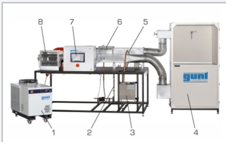
1 water chiller, 2 flow meter, 3 steam humidifier, 4 climatic chamber, 5 steam distributor (humidifier), 6 air cooler, 7 PLC, 8 outer air inlet with fan; covered: air heater
