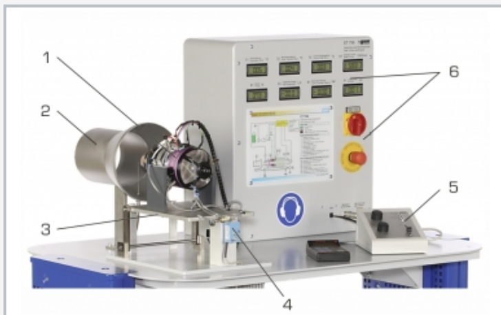
1 jet engine, 2 mixing pipe, 3 turbine platform, 4 force sensor for thrust measurement, 5 gas turbine controls, 6 displays and controls trainer
