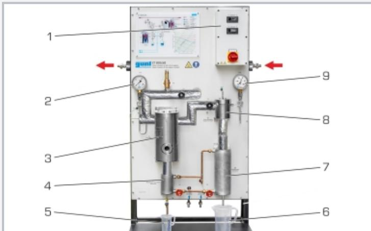
1 displays for temperature, 2 vapour inlet manometer, 3 cyclone water separator, 4 cooler for separated water, 5 measuring cup for separated water, 6 measuring cup for liquefied vapour, 7 condenser, 8 tank for depressurising the vapour, 9 manometer for depressurisation process; red: vapour inlet and outlet
