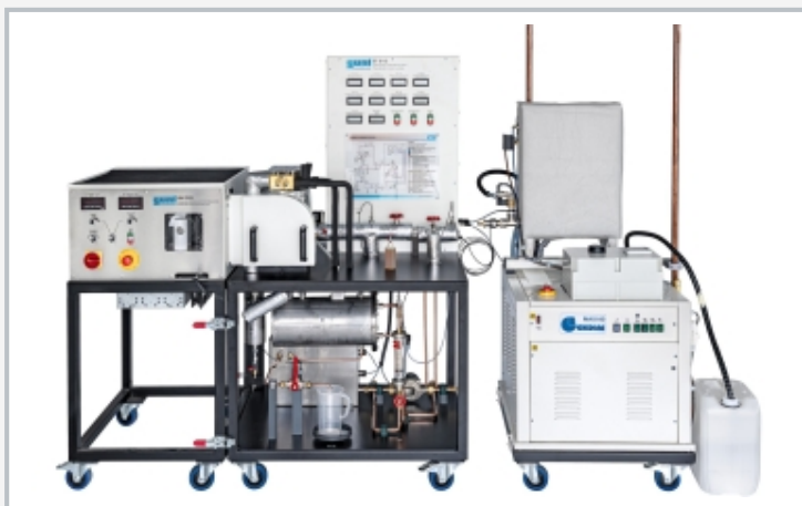
Experimental setup ready for operation: left: brake unit HM 365, centre: two-cylinder steam engine ET 813, right: steam generator ET 813.01
