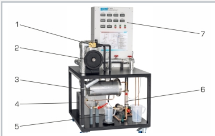
1 steam engine, 2 belt drive to HM 365, 3 condenser, 4 condensate tank, 5 condensate measuring tank, 6 sensor for cooling water flow rate, 7 displays and controls
