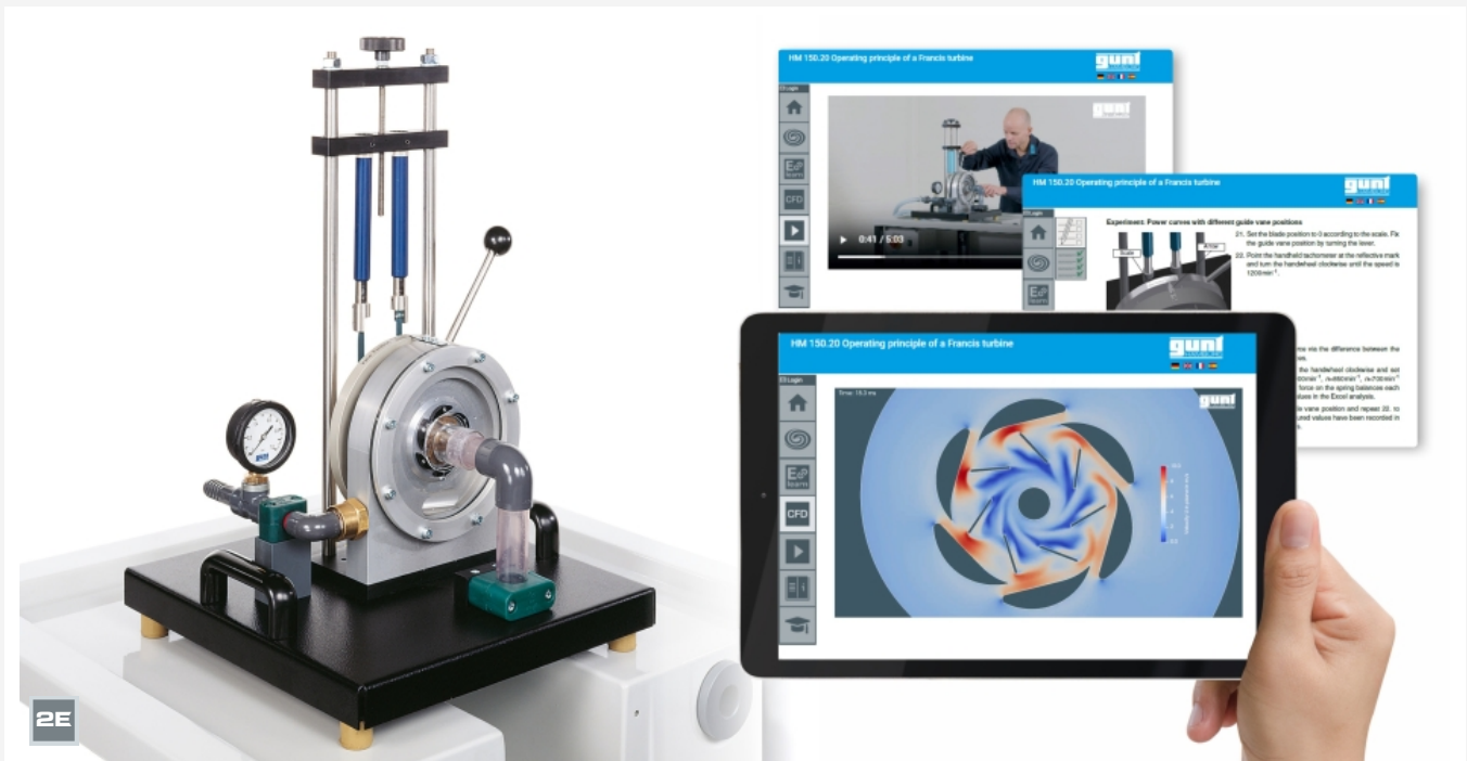
The illustration shows the experimental unit on the work surface of the HM 150 base module and the GUNT Science Media Center, tablet not included
