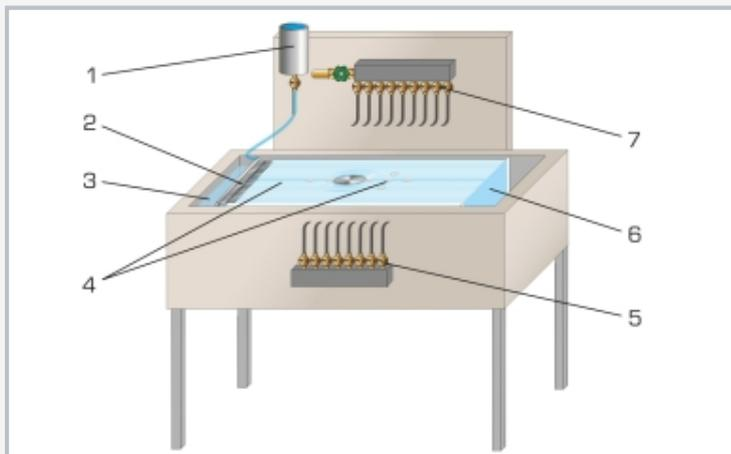
1 contrast medium, 2 nozzles for injecting the contrast medium, 3 water inlet, 4 Hele-Shaw cell with sources/sinks, 5 valves for sinks, 6 water outlet, 7 valves for sources
