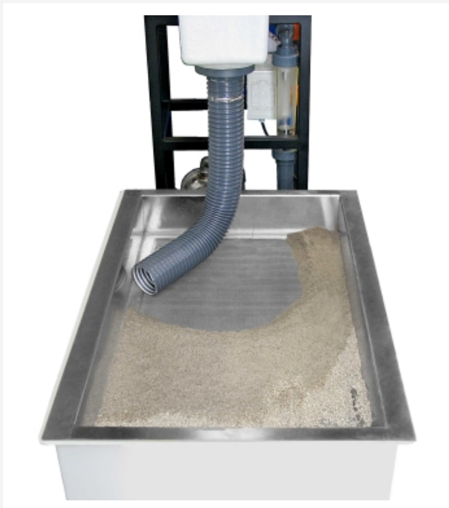
Sediment trap in the tank below the outlet element of HM 160.
