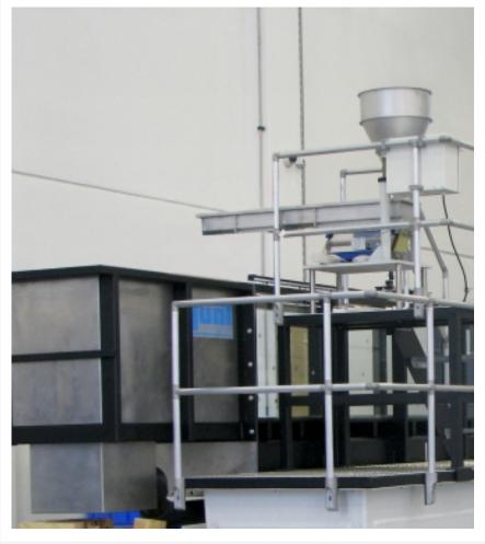
The illustration shows the sediment feeder on a platform.
