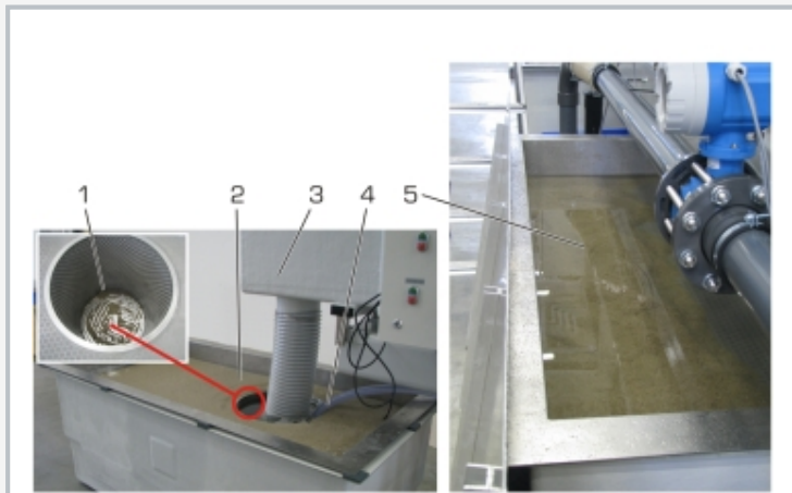
1 screen basket (pump not shown), 2 sediment, 3 outlet element of HM 162, 4 pipe system for transporting the mixture of water and sediment, 5 screen for sediment removal on second water tank
