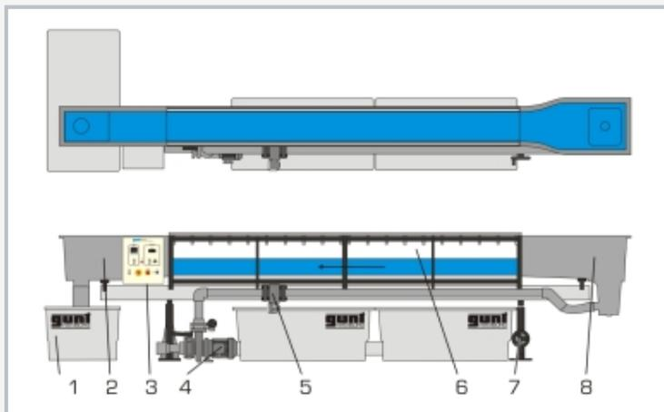
1 water tank, 2 outlet element, 3 switch box, 4 pump, 5 flow rate sensor, 6 experimental section, 7 inclination adjustment, 8 inlet element
