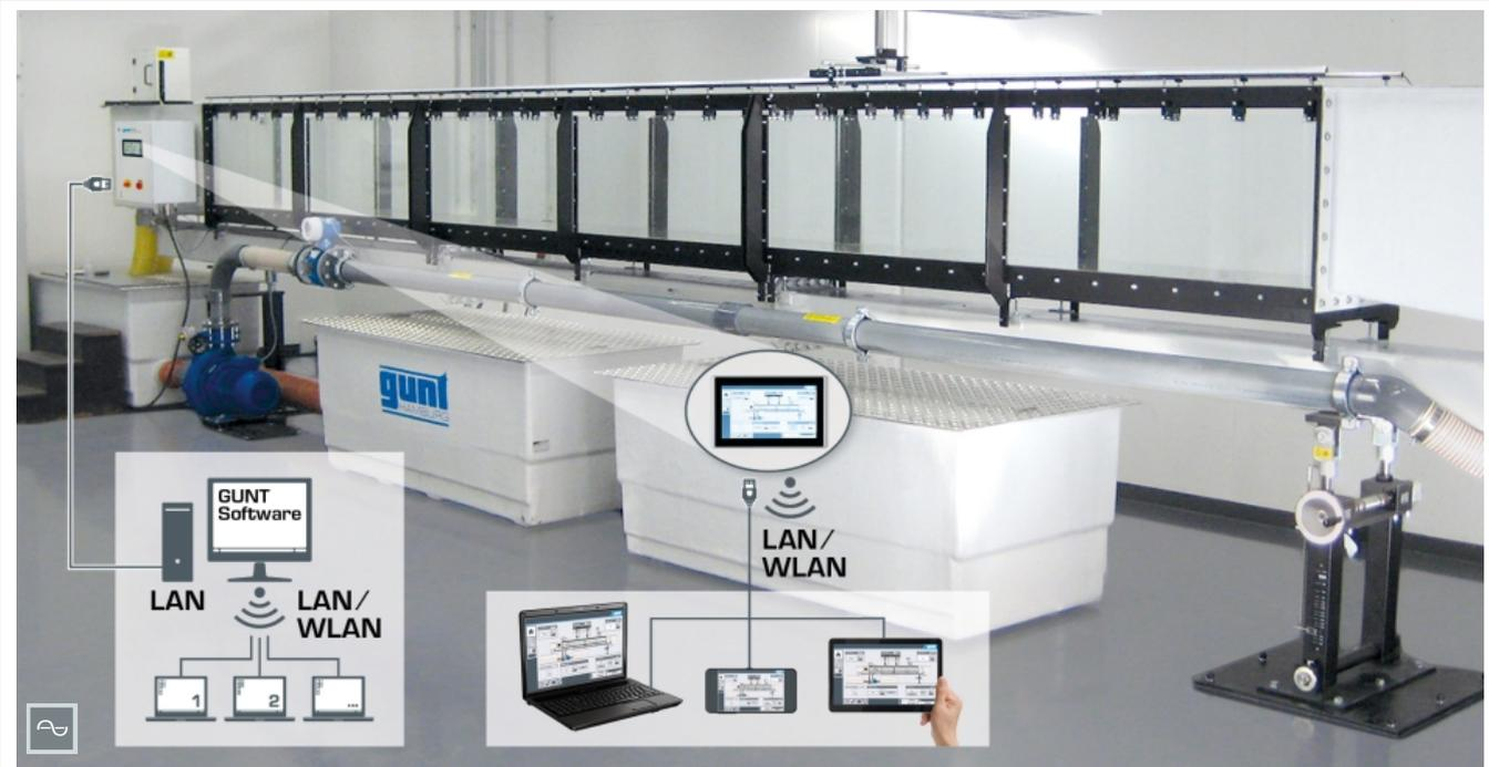
HM 163 (experimental section 7,5m) with the wave generator HM 163.41 and the level gauge HM 163.52, screen mirroring is possible on different end devices
