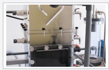
UASB reacor during experimental operation
