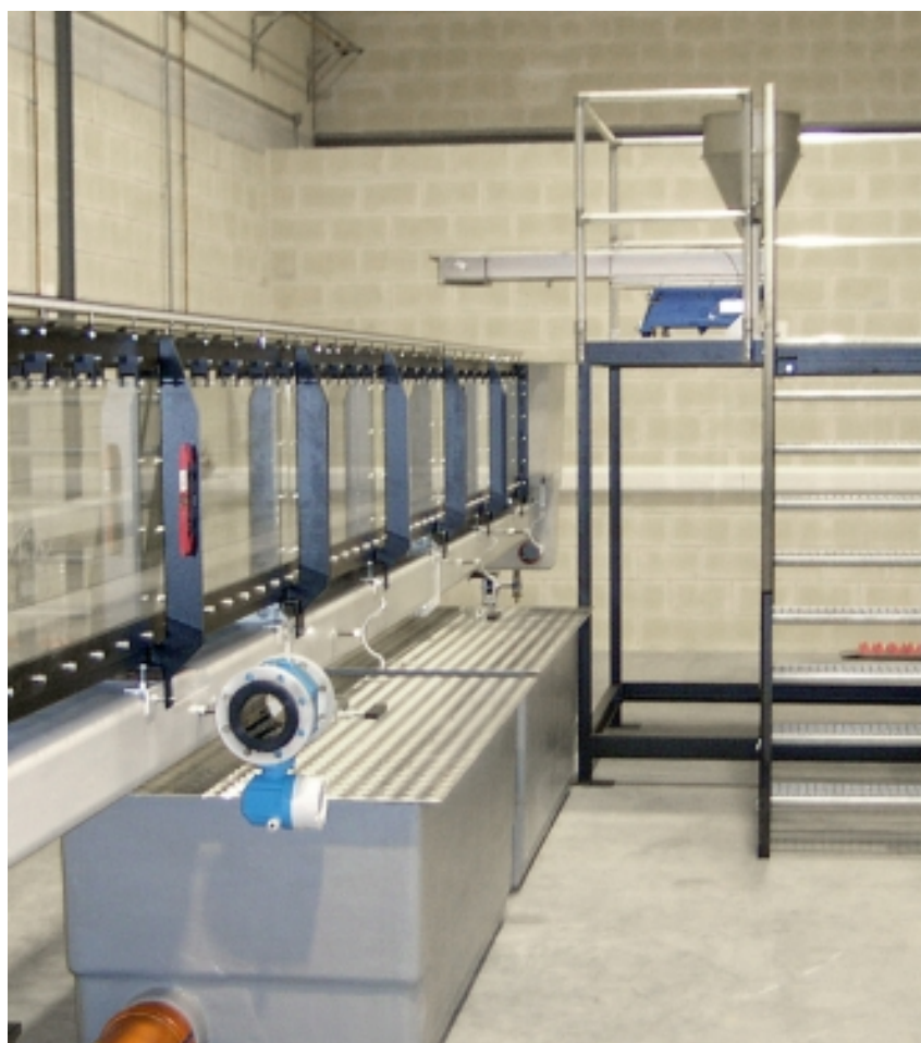
The illustration shows the sediment feeder on the platform.
