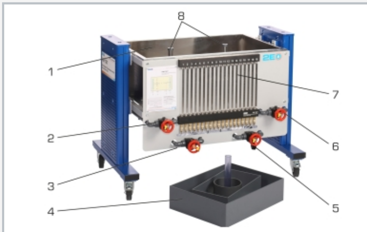
1 tank, 2 water supply, 3 water drain, 4 models, 5 water drain, 6 water supply, 7 tube manometers, 8 water drain via open-seam tube (well)
