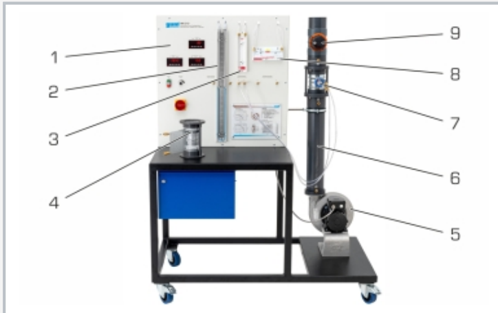
1 switch cabinet with display elements, 2 U-tube manometer, 3 single tube manometer, 4 Venturi nozzle, 5 radial fan with air intake, 6 pipe section, 7 iris diaphragm, 8 inclined tube manometer, 9 throttle valve
